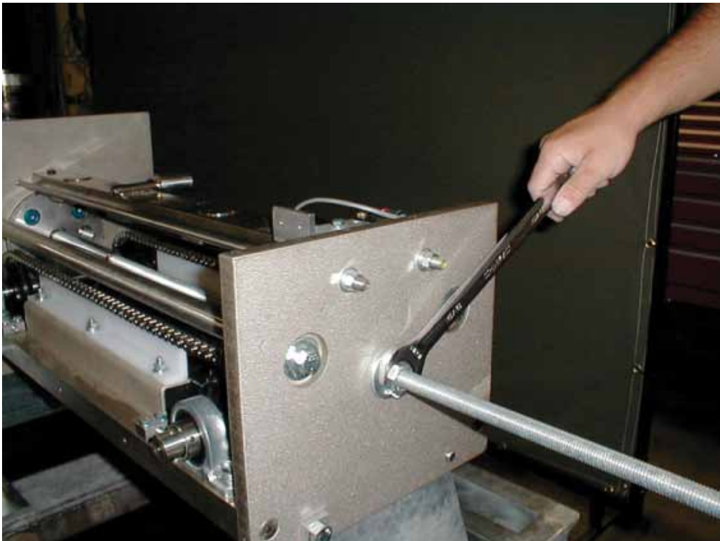
Figure 33: Piston Insertion into Flow Tube – Pulling Method Note: Refer to Table 15 for bolt torque values for assembling flow prover
