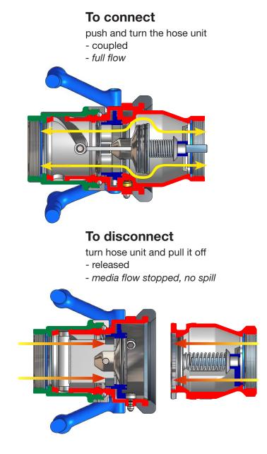
For the connection of DDCouplings, the hose unit (coupler) is pushed onto the tank unit (adapter).
